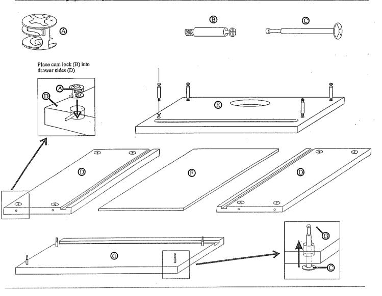
Turn cams clockwise about 1/2 a turn to lock the panels together.
