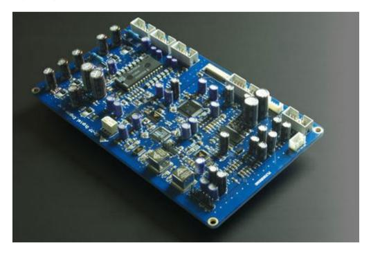
Trickling down from the AMR, the iGalvanic3.0 is the latest to receive a 'sprinkling' of Panasonic Os-Cons.
