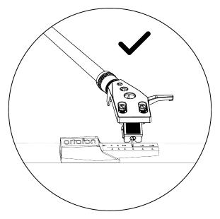
Adjust the counterweight until the stylus force gauge is in balance. Once the stylus is in balance, return the tonearm to its armrest. The anti-skate dial should be set to match the tracking force of the cartridge. Your factory-fitted cartridge has a tracking force of '2'.
