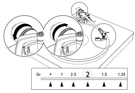
Adjusting the counterweight ensures the pressure the stylus applies to the record is correct. Too much pressure can cause distortion and lost information as well as wear to your records. Too little pressure and the stylus will jump and potentially damage your records.
