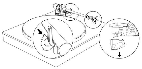
4. Place tonearm force gauge on the platter and carefully lower stylus onto "2"
