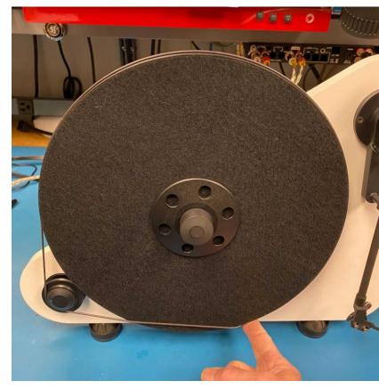
We will now hold the belt to the platter as shown and rotate the belt and platter until the belt is completely around platter and motor pulley.
