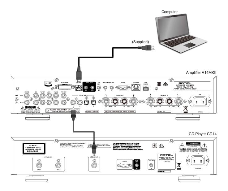
Figure 5: 12V Trigger Connections
