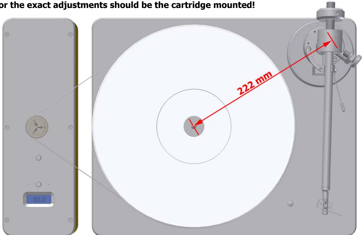
Picture 3: Distance from pivot to stylus
