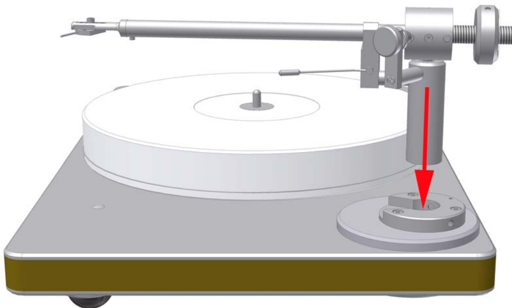
Picture 2: Putting the tonearm through the armboard
