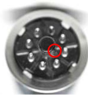
Guide pin shows on the bottom of a tube.
