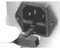
The fuse holder is released from the AC inlet.
