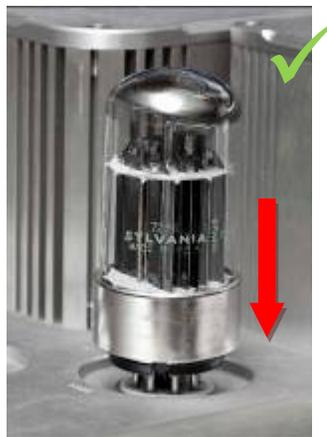
Insert a tube perpendicular to the socket.
