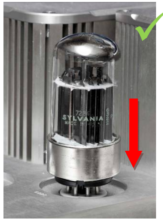
Insert a tube perpendicular to the socket.
