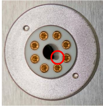
Tube socket guide pin indicator
