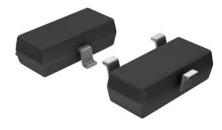
Computer matched pair complementary planar high gain bi-polar input transistors means 6dB lower output noise. The planar transistor is constructed by an etching and diffusion technique in which the junction is never exposed during processing, and the junctions reach the surface on one plane; characterized by very low leakage
